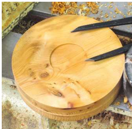
▲ Pic.8 The recess depth is 3mm, allowing the hole to be plugged with hardboard before the baize is applied. The chuck's sharp dovetail jaws will grip the shallow hole
